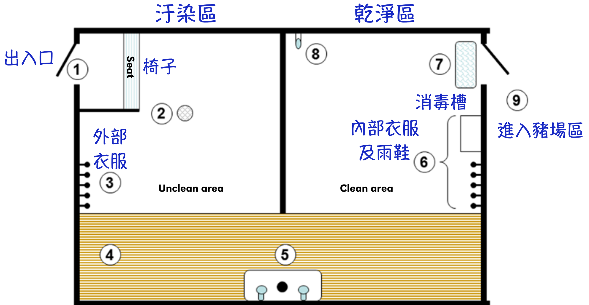
Figure 4. Danish entry method for a non-shower farm. 1. Only entrance to facility and footwear is removed; 2. Floor drain; 3. Street clothes are removed; 4. Wooden-grate passage is only entered in stocking feet; 5. Hands are washed and disinfected; 6. Protective clothing and boots; 7. Use footbath before entering unit; 8. Water-tap with hose; 9. Pig facility (adapted from Moore, 1992)
